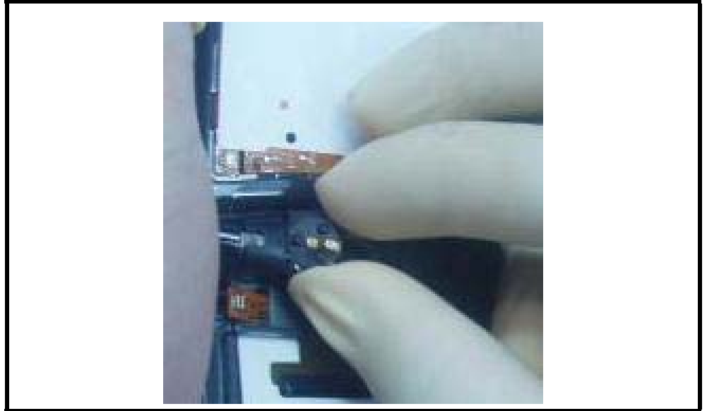
Figure 54. Installing the Vibrator Assembly
