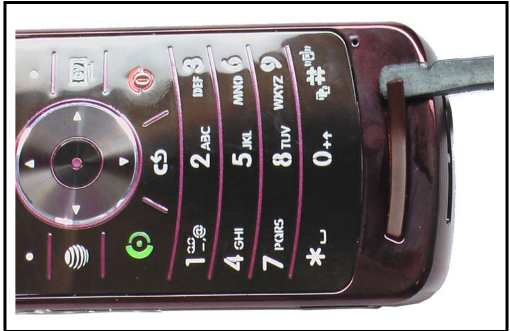
Figure 5. Removing the Bumper
