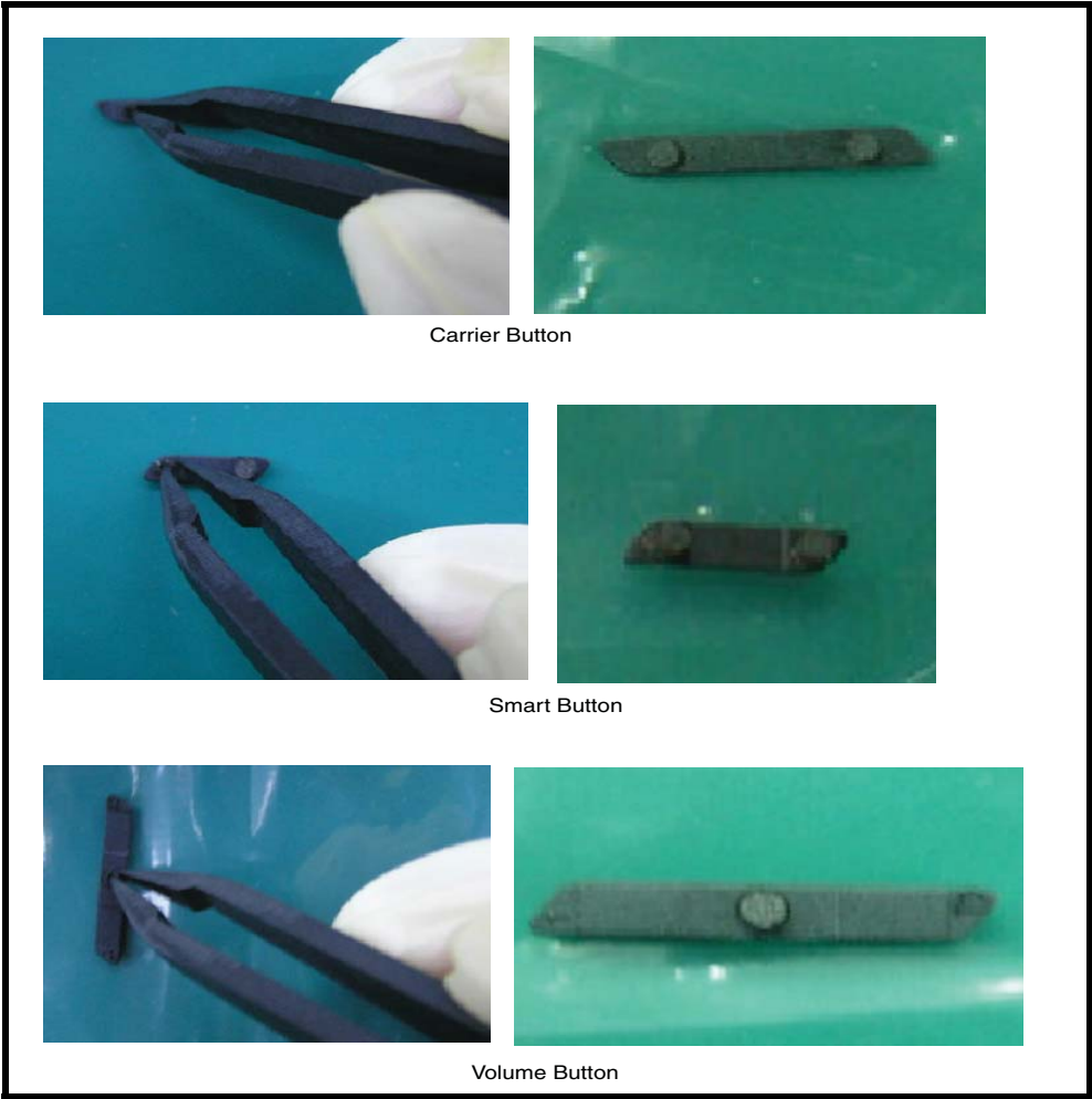
Figure 45. Installing the Side Key Pads
