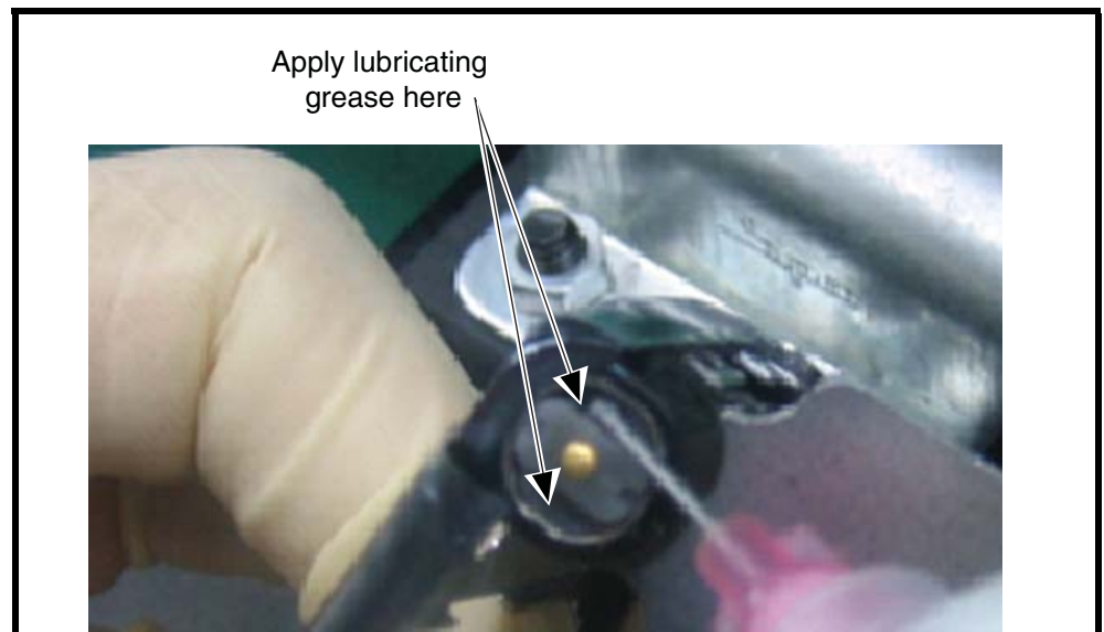
Figure 49. Lubricating the Flip Hinge
