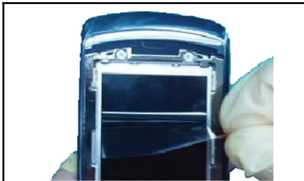
Figure 71. Removing the LCD Liner
