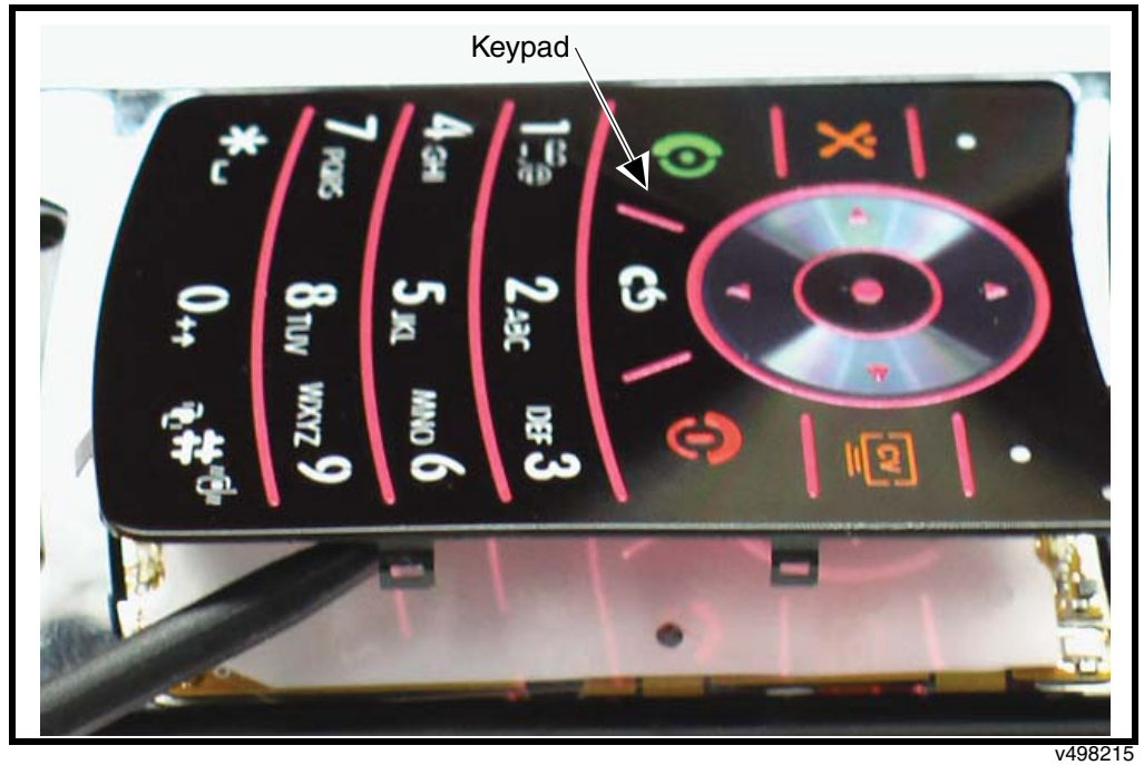
Figure 20. Placing the Keypad into the Front Housing
