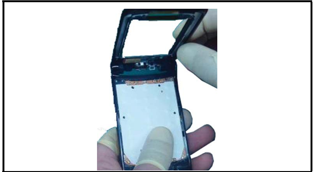
Figure 52. Inspecting the Flip Assembly
