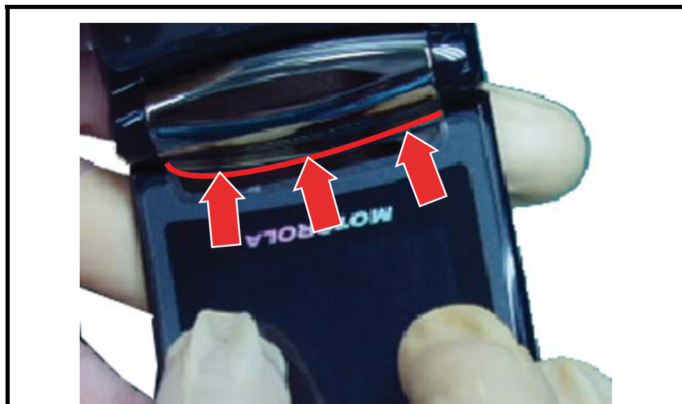
Figure 72. Attaching the Main Lens
